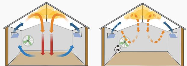
A system of circulation fans in the shed can be designed to bring hot air down from the ceiling to the floor (figure below), where it is needed to heat the floor and litter. Air speed that the circulation fans create at the litter surface will also evaporate more water from the litter. Circulation fans do not exhaust warm air out of the shed, so do not waste heat while moving the air. Exhaust fans still need to cycle on and off to remove moisture and ammonia from the shed and bring in fresh air.
