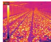
Thermal image before sprinkling (without cool-pads)
