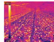
Thermal image in a neighbouring cool-pad shed (Images taken on Day 40. Temperature and relative humidity conditions were: ambient 28.8°C, 65% RH; in sprinkler shed 27.8°C, 70% RH; and in neighbouring shed with evaporative cooling pads 24.5 °C, 87% RH)
